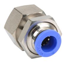
NITRA pneumatic push-to-connect fitting, bulkhead, nickel-plated brass body, nickel-plated brass threads, (1) R1/8 female BSPT to (1) 10mm push-to-connect. Package of 5.
