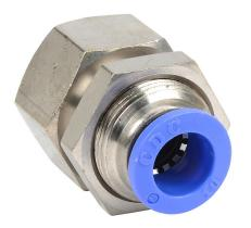
NITRA pneumatic push-to-connect fitting, bulkhead, nickel-plated brass body, nickel-plated brass threads, (1) R1/4 female BSPT to (1) 10mm push-to-connect. Package of 5.
