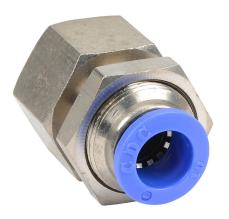
NITRA pneumatic push-to-connect fitting, female, bulkhead, nickel-plated brass body, nickel-plated brass threads, 10mm tube to R1/2 BSPT connection(s). Package of 5.
