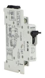
Eaton auxiliary contact, DPST contact(s), 2A @ 230VAC/0.5A @ 110VAC/VDC. For use with Eaton FAZ series supplementary protectors.
