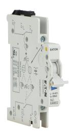
Eaton alarm/auxiliary contact, (2) SPDT contact(s), 2A @ 230VAC/0.5A @ 110VAC/VDC. For use with Eaton FAZ series supplementary protectors.
