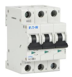
Eaton miniature supplementary protector, 8A, 480Y / 277 VAC / 96 VDC, 3-pole, D curve, thermal magnetic, 5kA @ 480Y/277 VAC interrupting rating, 35mm DIN rail mount.
