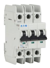
Eaton miniature circuit breaker, current-limiting, 8A, 480Y / 277 VAC / 96 VDC, 3-pole, D curve, thermal magnetic, 10kA @ 480Y/277 VAC interrupting rating, 35mm DIN rail mount.
