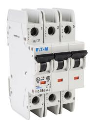
Eaton miniature circuit breaker, current-limiting, 8A, 240 VAC / 96 VDC, 3-pole, D curve, thermal magnetic, 10kA @ 240 VAC interrupting rating, 35mm DIN rail mount.
