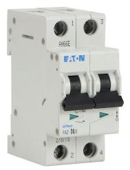
Eaton miniature supplementary protector, 8A, 480Y / 277 VAC / 96 VDC, 2-pole, D curve, thermal magnetic, 5kA @ 480Y/277 VAC interrupting rating, 35mm DIN rail mount.
