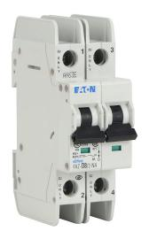
Eaton miniature circuit breaker, current-limiting, 8A, 480Y / 277 VAC / 96 VDC, 2-pole, D curve, thermal magnetic, 10kA @ 480Y/277 VAC interrupting rating, 35mm DIN rail mount.
