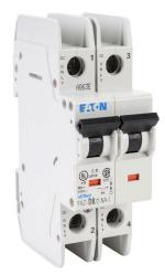
Eaton miniature circuit breaker, current-limiting, 8A, 240 VAC / 96 VDC, 2-pole, D curve, thermal magnetic, 10kA @ 240 VAC interrupting rating, 35mm DIN rail mount.
