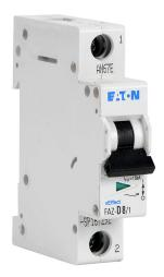
Eaton miniature supplementary protector, 8A, 277 VAC / 48 VDC, 1-pole, D curve, thermal magnetic, 5kA @ 277 VAC interrupting rating, 35mm DIN rail mount.
