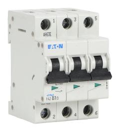
Eaton miniature supplementary protector, 7A, 480Y / 277 VAC / 96 VDC, 3-pole, D curve, thermal magnetic, 5kA @ 480Y/277 VAC interrupting rating, 35mm DIN rail mount.
