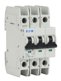
Eaton miniature circuit breaker, current-limiting, 7A, 480Y / 277 VAC / 96 VDC, 3-pole, D curve, thermal magnetic, 10kA @ 480Y/277 VAC interrupting rating, 35mm DIN rail mount.
