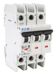
Eaton miniature circuit breaker, current-limiting, 7A, 240 VAC / 96 VDC, 3-pole, D curve, thermal magnetic, 10kA @ 240 VAC interrupting rating, 35mm DIN rail mount.
