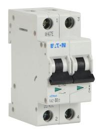
Eaton miniature supplementary protector, 7A, 480Y / 277 VAC / 96 VDC, 2-pole, D curve, thermal magnetic, 5kA @ 480Y/277 VAC interrupting rating, 35mm DIN rail mount.
