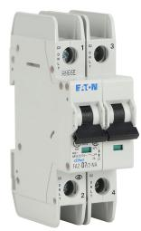
Eaton miniature circuit breaker, current-limiting, 7A, 480Y / 277 VAC / 96 VDC, 2-pole, D curve, thermal magnetic, 10kA @ 480Y/277 VAC interrupting rating, 35mm DIN rail mount.
