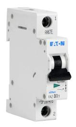
Eaton miniature supplementary protector, 7A, 277 VAC / 48 VDC, 1-pole, D curve, thermal magnetic, 5kA @ 277 VAC interrupting rating, 35mm DIN rail mount.
