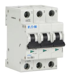
Eaton miniature supplementary protector, 6A, 480Y / 277 VAC / 96 VDC, 3-pole, D curve, thermal magnetic, 5kA @ 480Y/277 VAC interrupting rating, 35mm DIN rail mount.
