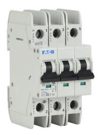
Eaton miniature circuit breaker, current-limiting, 6A, 480Y / 277 VAC / 96 VDC, 3-pole, D curve, thermal magnetic, 10kA @ 480Y/277 VAC interrupting rating, 35mm DIN rail mount.
