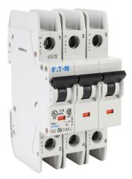
Eaton miniature circuit breaker, current-limiting, 6A, 240 VAC / 96 VDC, 3-pole, D curve, thermal magnetic, 10kA @ 240 VAC interrupting rating, 35mm DIN rail mount.
