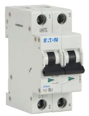
Eaton miniature supplementary protector, 6A, 480Y / 277 VAC / 96 VDC, 2-pole, D curve, thermal magnetic, 5kA @ 480Y/277 VAC interrupting rating, 35mm DIN rail mount.
