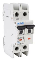
Eaton miniature circuit breaker, current-limiting, 6A, 240 VAC / 96 VDC, 2-pole, D curve, thermal magnetic, 10kA @ 240 VAC interrupting rating, 35mm DIN rail mount.
