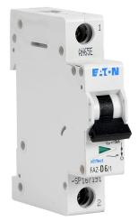
Eaton miniature supplementary protector, 6A, 277 VAC / 48 VDC, 1-pole, D curve, thermal magnetic, 5kA @ 277 VAC interrupting rating, 35mm DIN rail mount.
