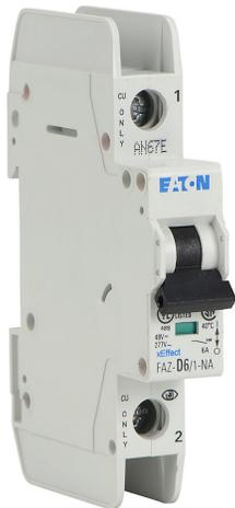
Eaton miniature circuit breaker, current-limiting, 6A, 277 VAC / 48 VDC, 1-pole, D curve, thermal magnetic, 10kA @ 277 VAC interrupting rating, 35mm DIN rail mount.
