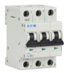
Eaton miniature supplementary protector, 5A, 480Y / 277 VAC / 96 VDC, 3-pole, D curve, thermal magnetic, 5kA @ 480Y/277 VAC interrupting rating, 35mm DIN rail mount.
