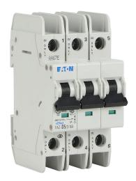
Eaton miniature circuit breaker, current-limiting, 5A, 480Y / 277 VAC / 96 VDC, 3-pole, D curve, thermal magnetic, 10kA @ 480Y/277 VAC interrupting rating, 35mm DIN rail mount.
