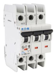
Eaton miniature circuit breaker, current-limiting, 5A, 240 VAC / 96 VDC, 3-pole, D curve, thermal magnetic, 10kA @ 240 VAC interrupting rating, 35mm DIN rail mount.
