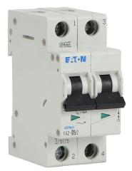
Eaton miniature supplementary protector, 5A, 480Y / 277 VAC / 96 VDC, 2-pole, D curve, thermal magnetic, 5kA @ 480Y/277 VAC interrupting rating, 35mm DIN rail mount.
