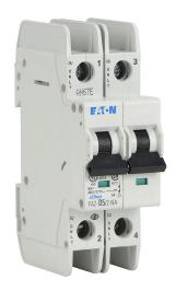
Eaton miniature circuit breaker, current-limiting, 5A, 480Y / 277 VAC / 96 VDC, 2-pole, D curve, thermal magnetic, 10kA @ 480Y/277 VAC interrupting rating, 35mm DIN rail mount.
