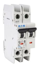
Eaton miniature circuit breaker, current-limiting, 5A, 240 VAC / 96 VDC, 2-pole, D curve, thermal magnetic, 10kA @ 240 VAC interrupting rating, 35mm DIN rail mount.
