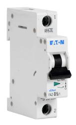
Eaton miniature supplementary protector, 5A, 277 VAC / 48 VDC, 1-pole, D curve, thermal magnetic, 5kA @ 277 VAC interrupting rating, 35mm DIN rail mount.
