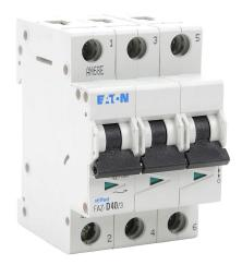
Eaton miniature supplementary protector, 40A, 480Y / 277 VAC / 96 VDC, 3-pole, D curve, thermal magnetic, 5kA @ 480Y/277 VAC interrupting rating, 35mm DIN rail mount.
