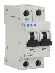
Eaton miniature supplementary protector, 40A, 480Y / 277 VAC / 96 VDC, 2-pole, D curve, thermal magnetic, 5kA @ 480Y/277 VAC interrupting rating, 35mm DIN rail mount.
