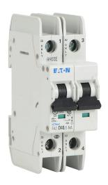
Eaton miniature circuit breaker, current-limiting, 40A, 240 VAC / 48 VDC, 2-pole, D curve, thermal magnetic, 10kA @ 240 VAC interrupting rating, 35mm DIN rail mount.
