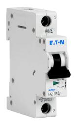
Eaton miniature supplementary protector, 40A, 277 VAC / 48 VDC, 1-pole, D curve, thermal magnetic, 5kA @ 277 VAC interrupting rating, 35mm DIN rail mount.
