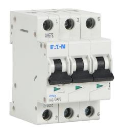
Eaton miniature supplementary protector, 4A, 480Y / 277 VAC / 96 VDC, 3-pole, D curve, thermal magnetic, 5kA @ 480Y/277 VAC interrupting rating, 35mm DIN rail mount.
