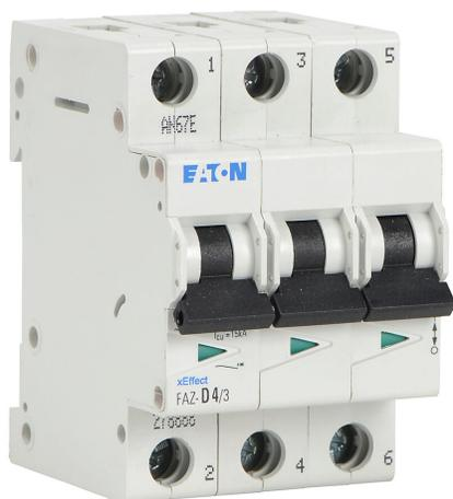
Eaton miniature supplementary protector, 4A, 480Y / 277 VAC / 96 VDC, 3-pole, D curve, thermal magnetic, 5kA @ 480Y/277 VAC interrupting rating, 35mm DIN rail mount.
