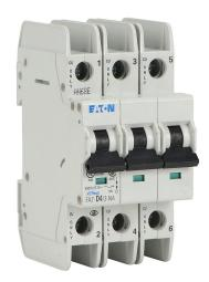
Eaton miniature circuit breaker, current-limiting, 4A, 480Y / 277 VAC / 96 VDC, 3-pole, D curve, thermal magnetic, 10kA @ 480Y/277 VAC interrupting rating, 35mm DIN rail mount.
