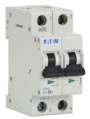
Eaton miniature supplementary protector, 4A, 480Y / 277 VAC / 96 VDC, 2-pole, D curve, thermal magnetic, 5kA @ 480Y/277 VAC interrupting rating, 35mm DIN rail mount.
