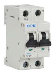
Eaton miniature supplementary protector, 4A, 480Y / 277 VAC / 96 VDC, 2-pole, D curve, thermal magnetic, 5kA @ 480Y/277 VAC interrupting rating, 35mm DIN rail mount.
