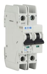
Eaton miniature circuit breaker, current-limiting, 4A, 480Y / 277 VAC / 96 VDC, 2-pole, D curve, thermal magnetic, 10kA @ 480Y/277 VAC interrupting rating, 35mm DIN rail mount.
