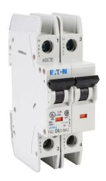
Eaton miniature circuit breaker, current-limiting, 4A, 240 VAC / 96 VDC, 2-pole, D curve, thermal magnetic, 10kA @ 240 VAC interrupting rating, 35mm DIN rail mount.
