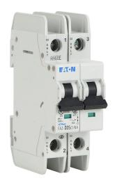
Eaton miniature circuit breaker, current-limiting, 35A, 240 VAC / 48 VDC, 2-pole, D curve, thermal magnetic, 10kA @ 240 VAC interrupting rating, 35mm DIN rail mount.
