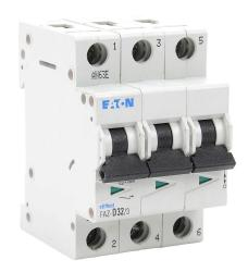
Eaton miniature supplementary protector, 32A, 480Y / 277 VAC / 96 VDC, 3-pole, D curve, thermal magnetic, 5kA @ 480Y/277 VAC interrupting rating, 35mm DIN rail mount.
