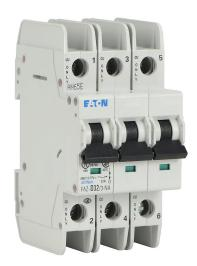
Eaton miniature circuit breaker, current-limiting, 32A, 480Y / 277 VAC / 96 VDC, 3-pole, D curve, thermal magnetic, 10kA @ 480Y/277 VAC interrupting rating, 35mm DIN rail mount.
