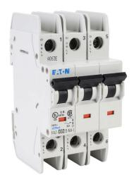
Eaton miniature circuit breaker, current-limiting, 32A, 240 VAC / 96 VDC, 3-pole, D curve, thermal magnetic, 10kA @ 240 VAC interrupting rating, 35mm DIN rail mount.
