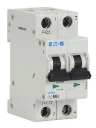
Eaton miniature supplementary protector, 32A, 480Y / 277 VAC / 96 VDC, 2-pole, D curve, thermal magnetic, 5kA @ 480Y/277 VAC interrupting rating, 35mm DIN rail mount.
