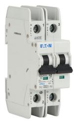
Eaton miniature circuit breaker, current-limiting, 32A, 480Y / 277 VAC / 96 VDC, 2-pole, D curve, thermal magnetic, 10kA @ 480Y/277 VAC interrupting rating, 35mm DIN rail mount.
