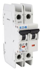
Eaton miniature circuit breaker, current-limiting, 32A, 240 VAC / 96 VDC, 2-pole, D curve, thermal magnetic, 10kA @ 240 VAC interrupting rating, 35mm DIN rail mount.
