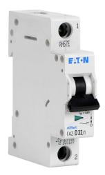
Eaton miniature supplementary protector, 32A, 277 VAC / 48 VDC, 1-pole, D curve, thermal magnetic, 5kA @ 277 VAC interrupting rating, 35mm DIN rail mount.
