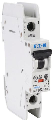
Eaton miniature circuit breaker, current-limiting, 32A, 240 VAC / 48 VDC, 1-pole, D curve, thermal magnetic, 10kA @ 240 VAC interrupting rating, 35mm DIN rail mount.
